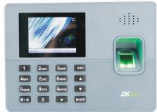
**k60** is a fingerprint time & attendance and access control terminal, which can connect with third electric lock, exit button, The 2.8 inch TFT screen can display more information vividly, including fingerprint image and verification result etc. TCP/IP communication is a standard function which makes sure the data transmission between terminal and PC can be easily done within several seconds. It's an ideal product for SMB market.
